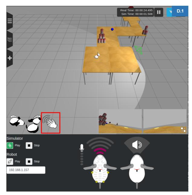
Once MiRo has finished the movement, the code will enter the while loop where it is waiting for a change in the state of MiRo's body touch sensors. As we cannot physically touch the simulated MiRo, we need to use another interaction button. Press the Body Stroke icon (highlighted in red in D.2).
